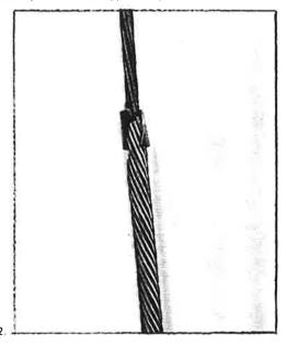
To achieve maximum coverage with the end sleeve, the application should be conducted in the following manner. Place the slot side of the end sleeve over the long leg of the dead-end.
